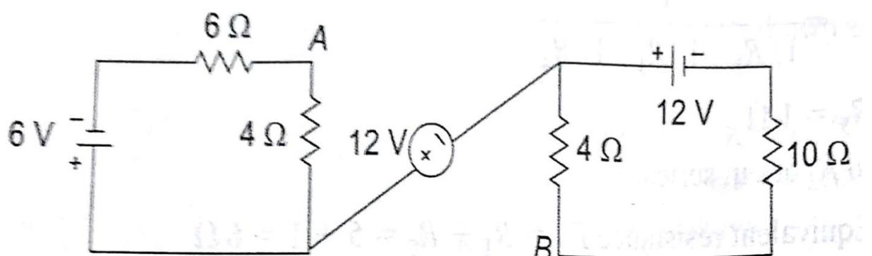
8. a) Find the voltages at node1 and node2 by using node analysis
